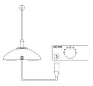
3. Microphone detachment: Press the release tab of the XLRF-type socket on the microphone stand and pull out the microphone.
