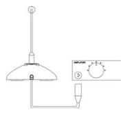
3. Microphone detachment: Press the release tab of the XLRF-type socket on the microphone stand and pull out the microphone.
